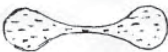
Figure 2 : Cross-section of the squeezed tube in approximately 9 m height, after the water level has fallen to 10 m.
