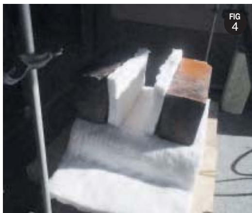
Figure 4: The ceramic fibre lining of the sides of the fire box, which must be just big enough to fit the steel calcination tube with only small gaps around it.
