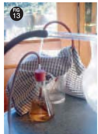
Figure 12: The working kiln with the burner going and a glass tube extending from the calcination tube taking the vented gases through the conical flask containing dilute red cabbage juice.
