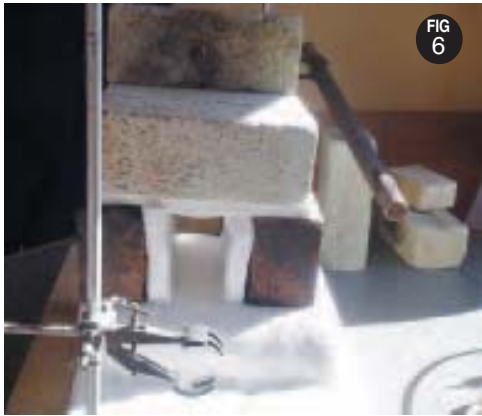
Figure 6: The addition of the roof bricks on to the ceramic fibre top.
