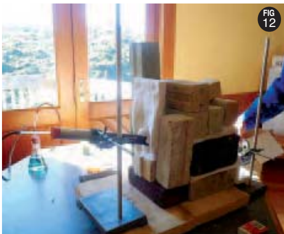
Figure 12: The working kiln with the burner going and a glass tube extending from the calcination tube taking the vented gases through the conical flask containing dilute red cabbage juice.
