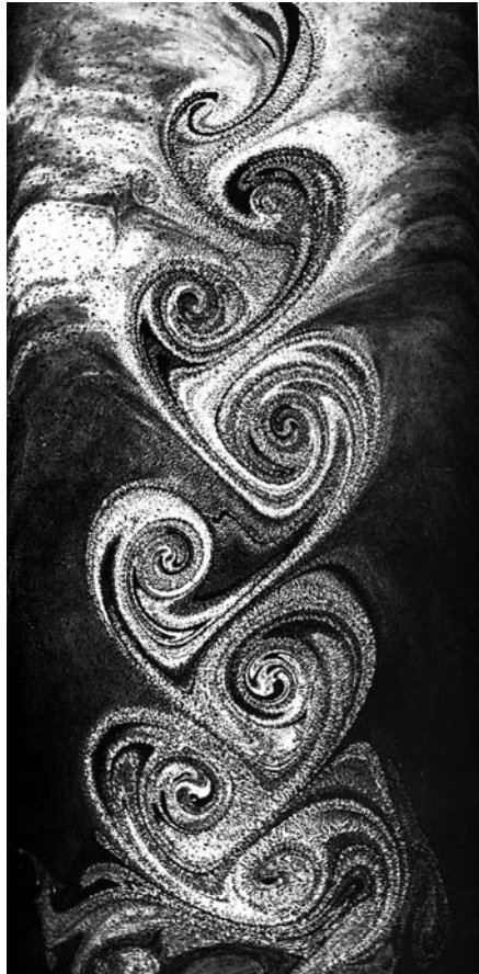
Vortice train created by drawing a feather through water on which has been sprinkled lycopodium powder from the spore cases of club mosses
